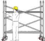
Install the platform with hatch on 4th rung of the five rung ladder frame.
