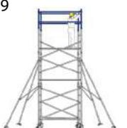
Erect guardrails and horizontal braces. Guardrails should be 0.5m and 1.0m above the platform in all cases.
