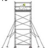
Move the second platform with hatch onto the 3rd rung of the 3 or 5 rung ladder frames. Fit toeboards to all working platforms.
