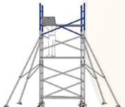
Add next lift of 3 or 5 rung ladder frames & next diagonal braces. Add next platform with hatch onto the 1st rung of 3 or 5 rung ladder frames.
