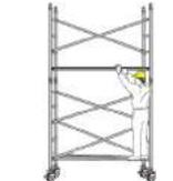
Move the platform with the hatch onto 1st rung of the 3 or 5 rung ladder frames.
