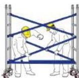
Install diagonal braces as shown. Ensure scaffold is level & plumb using a spirit level. Frame will now be self supporting.
