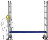
Position the ladder frame as shown. Lock the wheels, and clip the horizontal braces onto the rungs.
