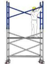
Add next lift of 3 or 5 rung ladder frames & next diagonal braces. Do not climb the platform until fully guardrailed.
